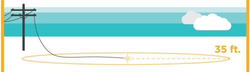
Downed power lines can energize the ground up to **35 feet** away—so keep your distance.
